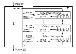
This approach is just a standard hardware technique, pipelining; it is possible because the protocol is naturally staged.
