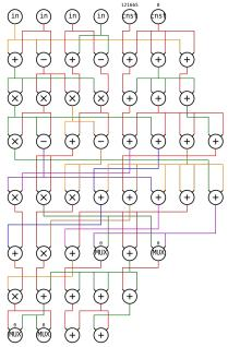
$\mathcal{P}$  executing AC: layers are sequential, but all gates at a layer can be executed in parallel
